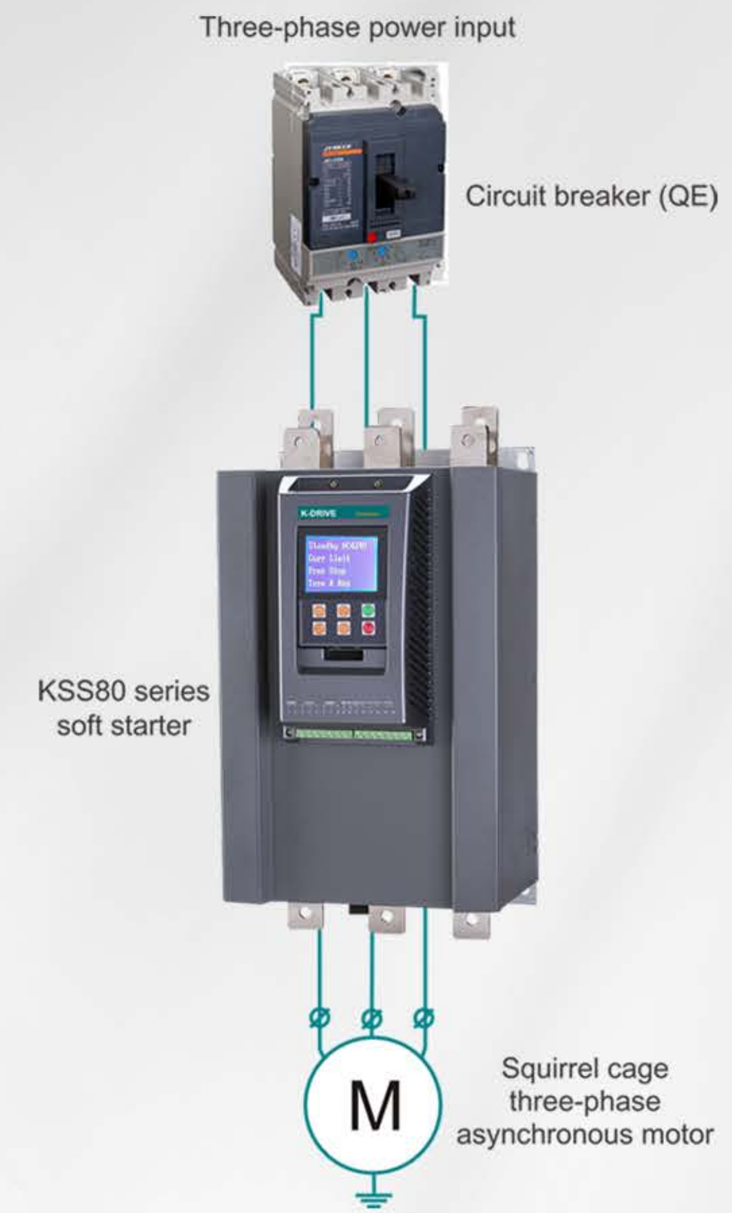
OUTER BYPASS SOFT STARTER CONNECT WAY
