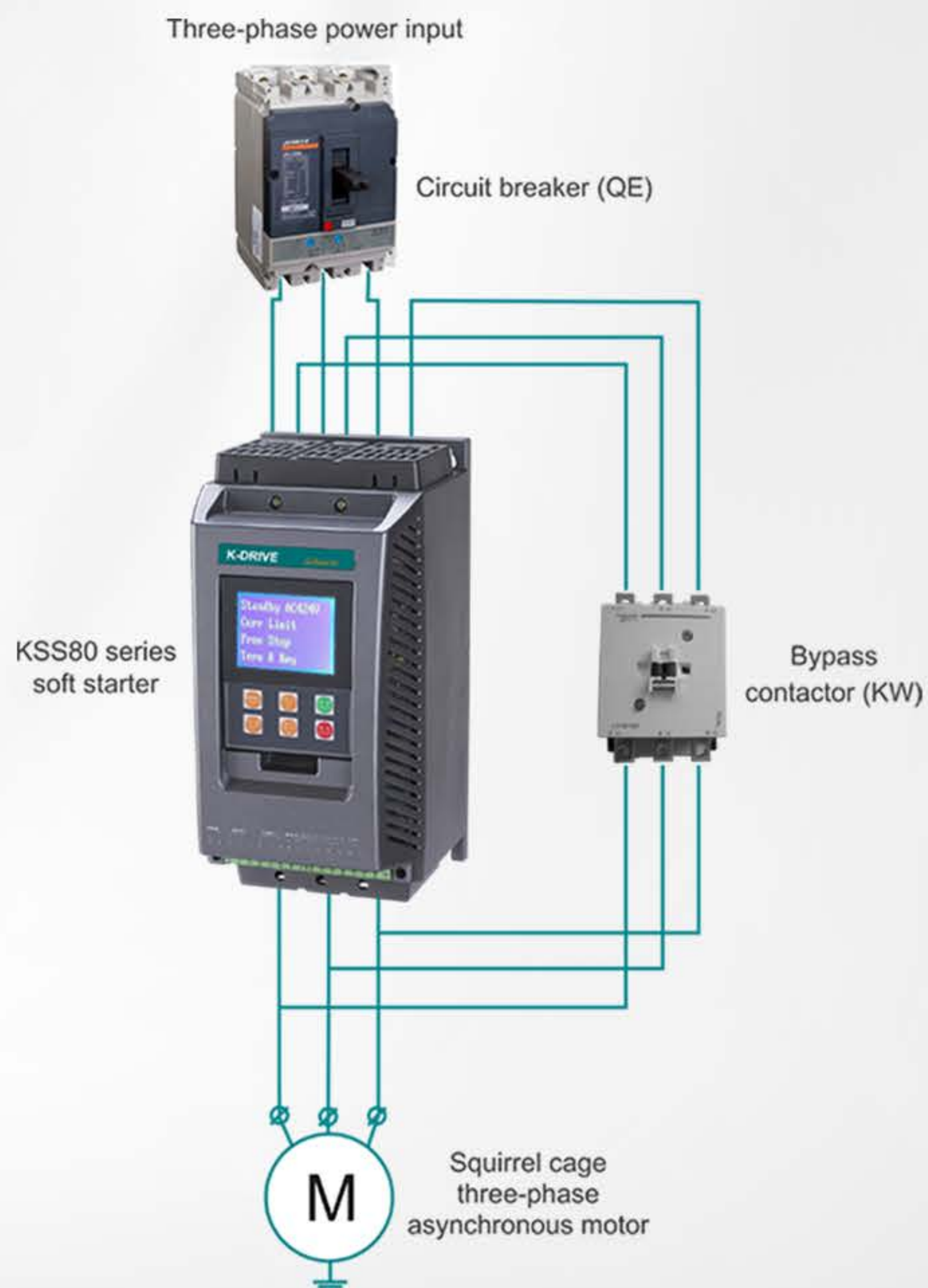
OUTER BYPASS SOFT STARTER CONNECT WAY
